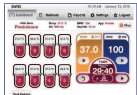
Dashboard screen when wireless in-shaft temperature sensors are Enabled
