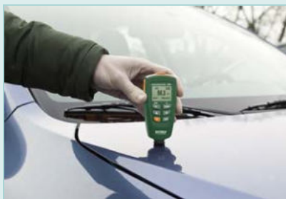
Measuring the thickness of automotive paint
