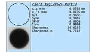
Image of a spherical metal powder particle
