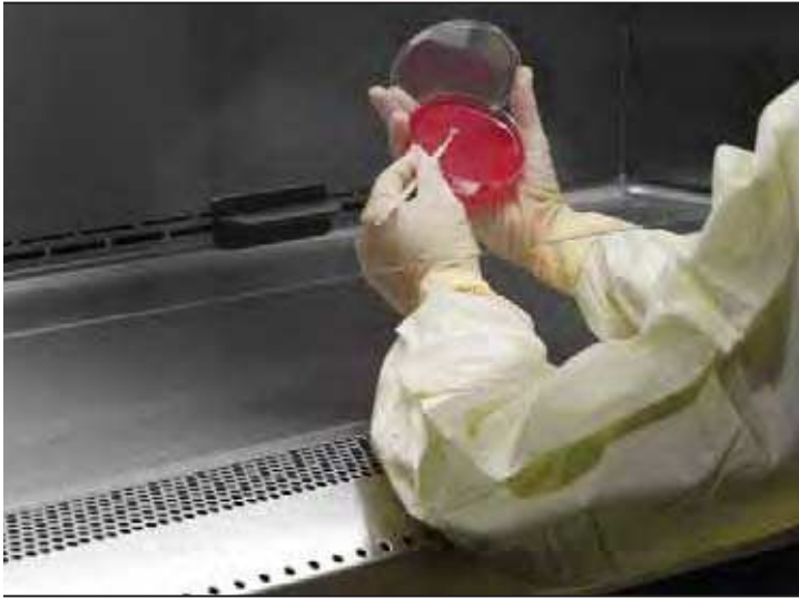
The curved inlet grille provides a comfortable surface for forearms resting on it. No additional armrest is needed. Reserve-Air™ Inflow Slots draw air into the cabinet should the operator inadvertently block portions of the inlet grille, maintaining safe airflow.
