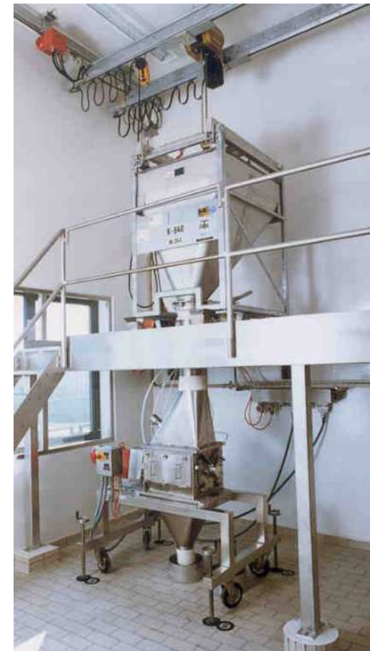
ESCO-Labor- Processing-Plant EL6 with extrude device and bottom outlet valve special edition for pasty products
