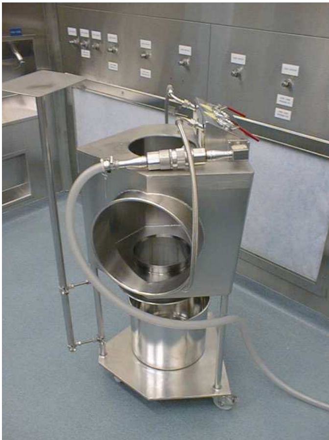
ESCO-Labor- Processing-Plant EL6 with extrude device and bottom outlet valve special edition for pasty products
