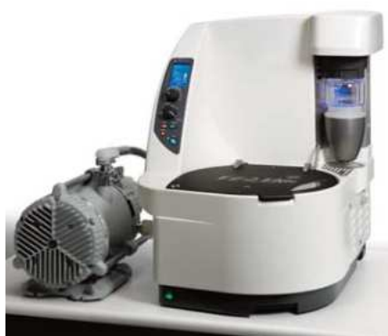
The Scroll pump used with the EZ-2 Elite delivers deeper vacuum than the diaphragm pumps found in the EZ-2 Standard, Envi and Plus.
