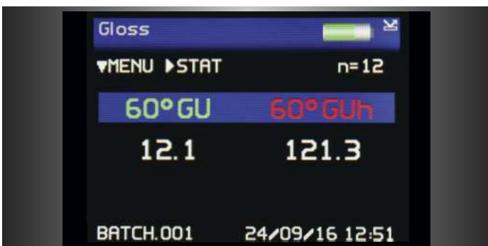
Pass / fail parameters can be defined for instant identification of non-conformances.
