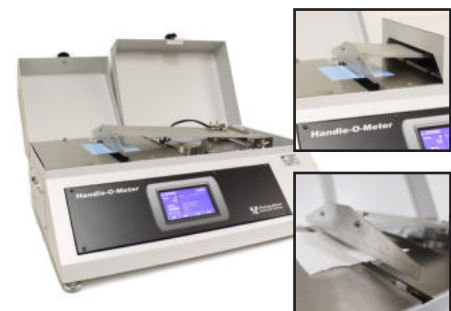
The Handle-O-Meter measures the combined effects of flexibility and surface friction of sheeted materials.
