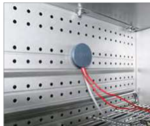
Access port with silicone plug
