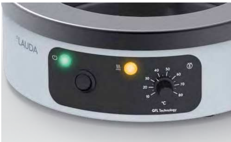
Adjustable bath temperature with heating activity display
