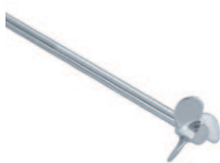
R 1381 Propeller stirrer, 3-bladed Flow-efficient design. For drawing the material to be mixed from the top and bottom. Minimum shearing forces. Used at medium to high speeds. Ident. No. 0001296000
