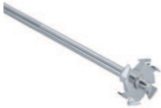
R 1303 Dissolver stirrer Radial flow, for drawing the material to be mixed from the top and bottom. High turbulence, high shearing forces. Particle reduction. Used at medium to high speeds. Ident. No. 0002746700
