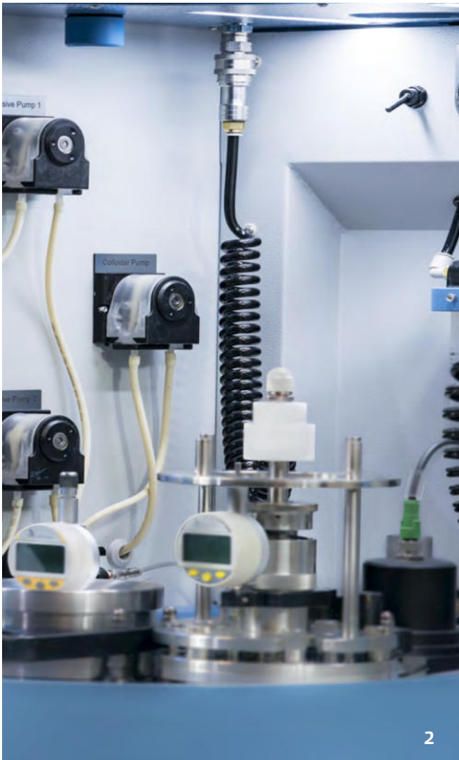
1: PM6 Precision Lapping & Polishing System 2: Metered abrasive feed unit via peristaltic pumps 3: Bluetooth enabled automatic plate flatness monitor 4: Integrated sample cleaning with de-ionised water and nitrogen gun
