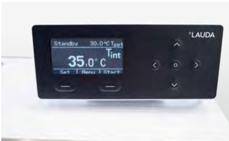
Low device height and 360° accessibility of the bath thanks to detachable remote control
