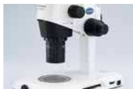
Slim LED transmitted light illuminator SZX2-ILLT
