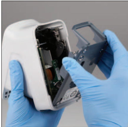
6. After the base has dried, reattach it to the analyzer and ensure it is locked into place.
