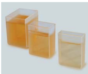
Measurement of liquid samples in square cells
