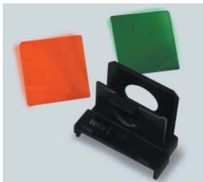
Measurement of transparent samples by setting on a sample clamp
