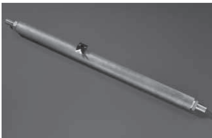
Figure 8.8: Measurement tube for the gas throughput
