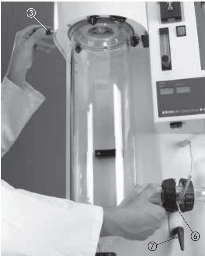
Figure 4.3: Installation of the spraying cylinder
