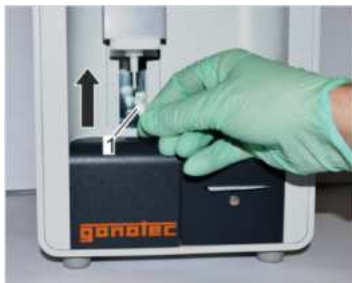
Fig. 82: Position measurement vessel
