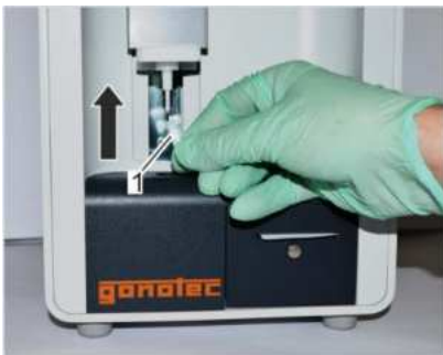
Fig. 146: Position measurement vessel
