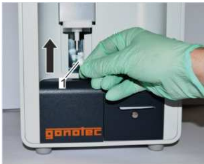
Fig. 19: Position measurement vessel
