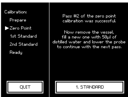
Fig. 72: Calibrate device using calibration standard
