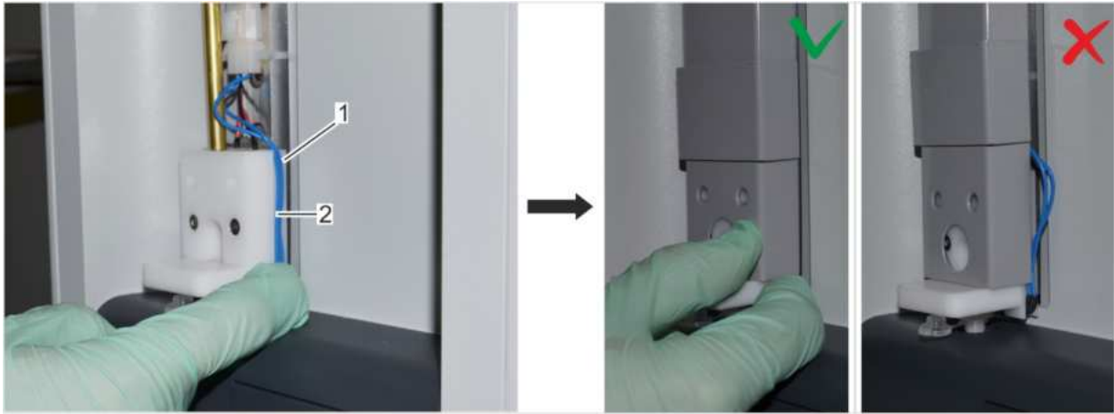
Fig. 108: Elevator cover with correct cable routing
