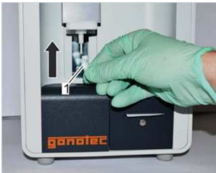
Fig. 64: Position measurement vessel
