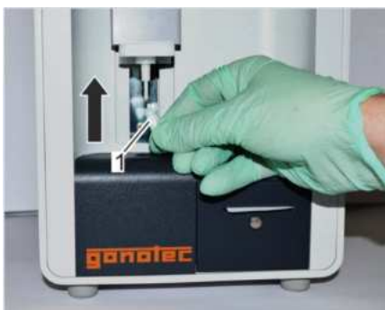
Fig. 70: Position measurement vessel
