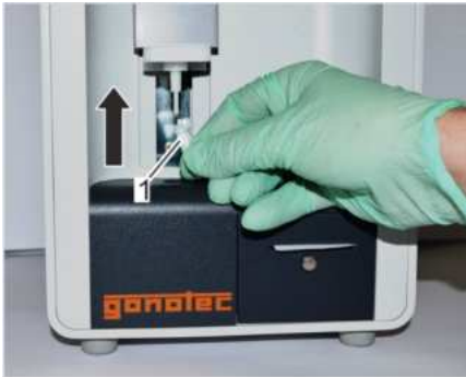
Fig. 94: Position measurement vessel
