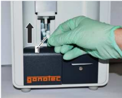
Fig. 52: Position measurement vessel
