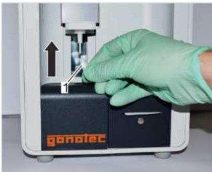
Fig. 128: Position measurement vessel
