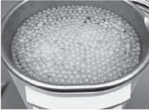
Fig. 5.2: Floating balls in the heating bath medium and cover for heating bath
