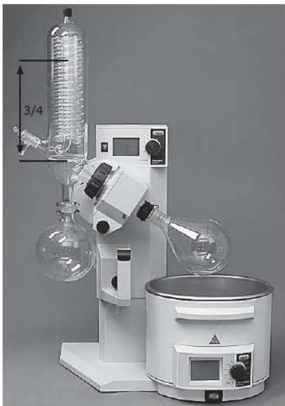
Fig. 6.6: Optional condensation area of a condenser
