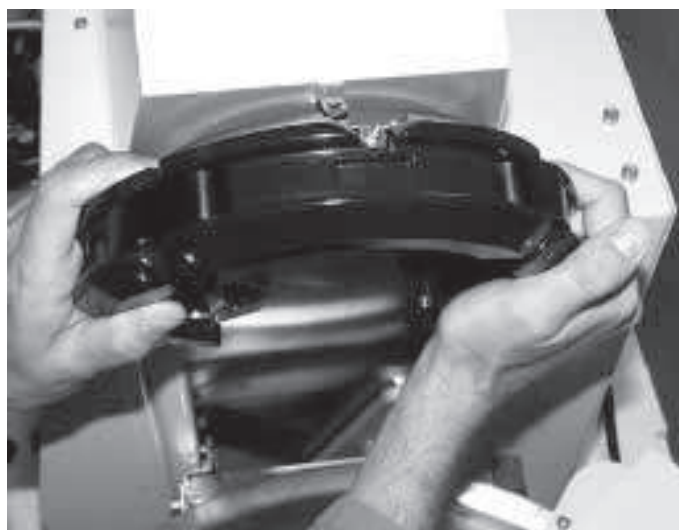
Fig. 25: Assembling the snap flange coupling
