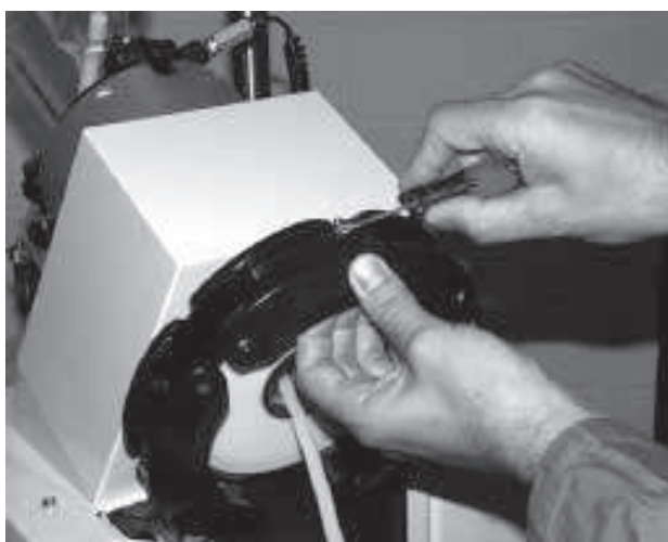
Fig. 24: Snap flange coupling, closed
