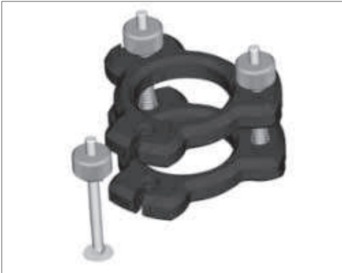
Fig. 4: Attachment of the EasyClamp
