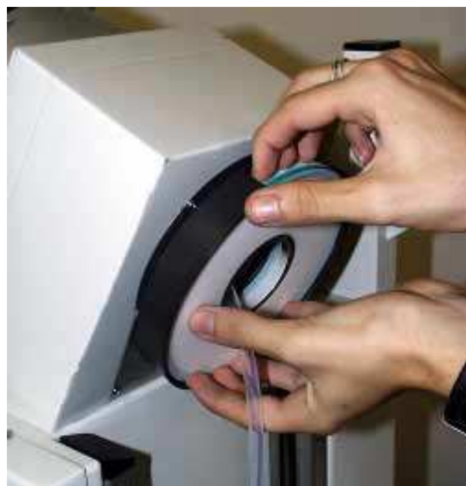
Fig. 26: Removing the evaporating flask seal
