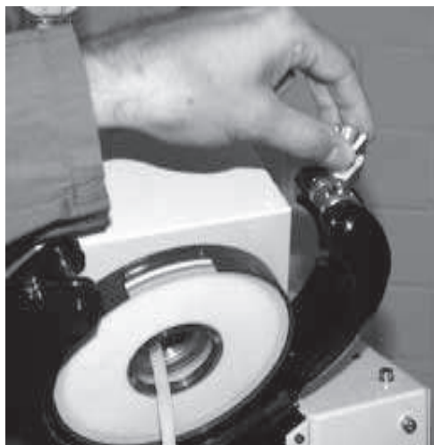
Fig. 14: Adjusting the tension on the closure
