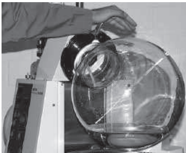
Fig. 13: Closing the snap flange coupling
