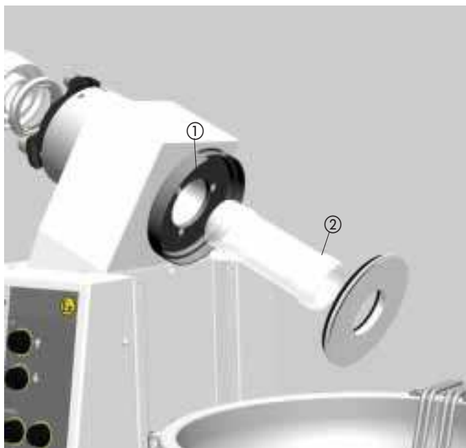
Fig. 27: Inserting the evaporating flask seal 1
